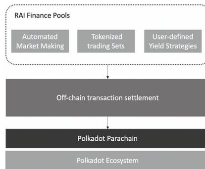
The protocol architecture provides layering for secure off-chain transactions with on-chain settlements to enable complex computations and more efficient transactions without losing the security and decentralization of blockchain. This increased complexity and speed can provide opportunities for market making and automated trading that are traditionally exclusive to centralized exchanges.
